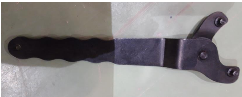
Figure 1. Customer delivered a tool for installing the post installed support ring.
